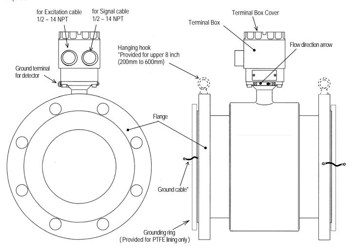
Figure 3.1.2 Appearance of Detector GF632
